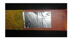
44 4 Use the aluminium foil to mend the slit as needed, leaving only 1 to 2 millimeters of open space for light to enter the slit. If the slit is too narrow, the spectra will appear dim. If the slit is too broad, the spectra will appear blurry.
