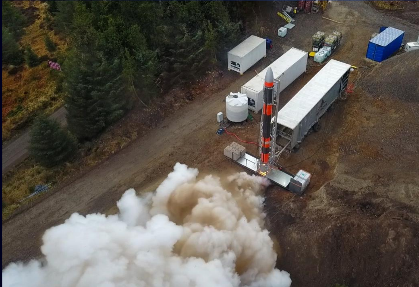
Skylark L's successful full static fire test using Skyrora's mobile launch complex in May 2020
