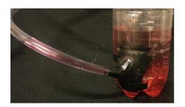
You will notice that when the water level in the plastic tubing is low, this is due to high air pressure experienced at lower elevations. However, when the water level in the plastic tubing is above the water level in the plastic bottle, then a low pressure is in effect due to higher elevations.
