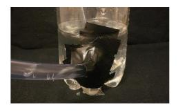
STEP 4 Using the tape, attach the plastic tubing to the top of the bottle, making sure you do not put pressure on the tubing. Then screw the lid back on to the top of the bottle.
