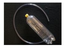
Insert the plastic tubing until the tip is halfway into the plastic bottle and is resting at the bottom of the bottle. Remember: it must be a tight fit.
